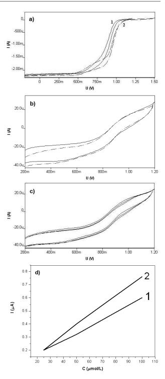
Fig. 2 Cyclic voltammograms obtained at 1mm Pt electrode at v = 50 mV/s.
