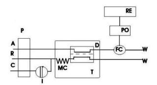
Fig. 1 Schematic presentation of the FIA aparatus used for amperometric determination of bromide content. A – acceptor solution; R – reagent; C – carrier; P – peristaltic pumps; I – injection valve; MC – mixing coil; D – gas-diffusion unit; FC – flow electrochemical cell; PO – potentiostat; RE – writer; T – thermostat; W – waste.
